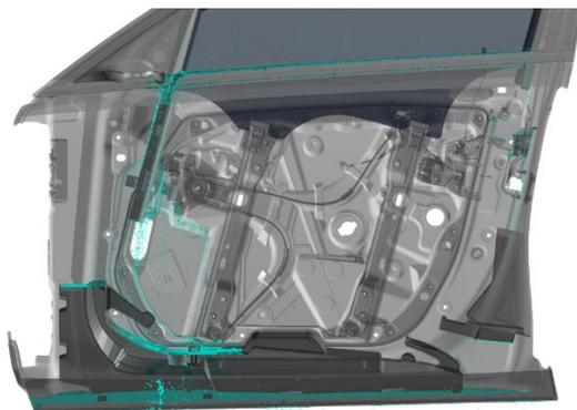
Image A: Flow path through a car door
