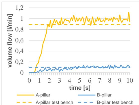
Comparison of volume flow rates computed with PreonLab and flow rates measured at the test bench.
