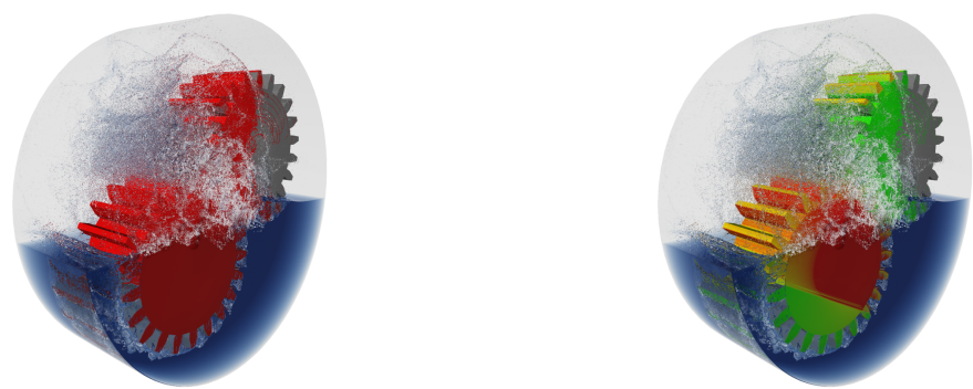
Figure 64: A gear setup after a simulation time of 0.2s. The gears start rotating after 0.1s. The wetting sensor in the left picture visualizes accumulated wetting whereas the wetting sensor in the right picture visualizes the wetting time. For the latter, the color legend is as follows: Green: > 0.0s, Yellow: 0.1s, Red: ≥ 0.2s.
